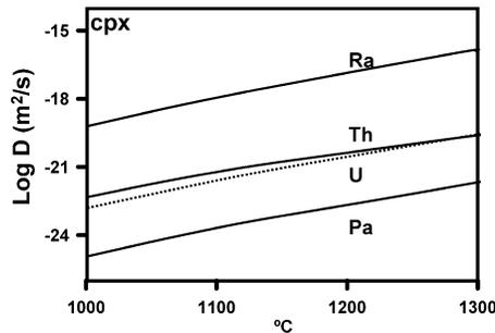
**Figure 4.** Diffusivities of Ra and Pa, calculated from elastic strain modeling, for clinopyroxene, based on Van Orman et al. (2001). Ra values are similar to those reported by Saal and Van Orman (2004). Diffusivities for U and Th are from Van Orman et al. (1998).
